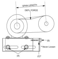
Tension new belts at the max. deflection force recommended for the belt section. Check the belt tension at least two times during the first 24 hours of operation. Any re tensioning should fall between the min. and max. deflection force values.
